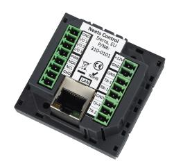
Easy to program. All Neets controllers are quickly programmed using Windows-based Neets Project Editor software. Even the most complex AV control systems can be configured in minutes using an intuitive graphical interface. You can program additional rooms with identical controls in a matter of seconds by simply using copy and paste. Programs are loaded via LAN, RS-232 or front-panel USB port.
