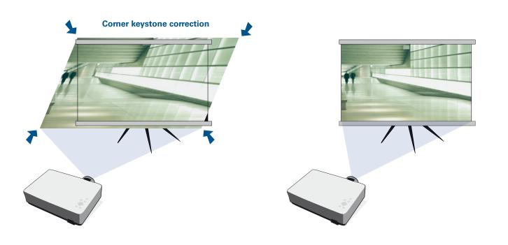
As the image corners can be individually adapted to the projection area – e.g. a screen – an accurate and sharp image is obtained even from unfavourable positions.
