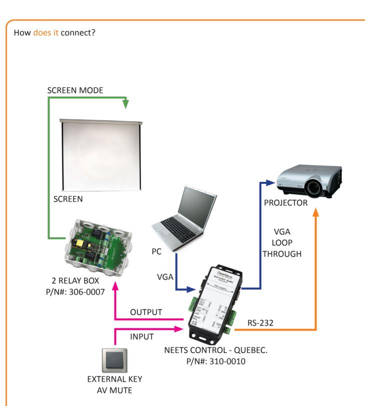
The Neets Control - QueBec detects a VGA signal from the PC and sends the signal through to the projector. Furthermore the Neets Control - QueBec sends a RS-232 signal to the projector. The Neets Control - QueBec controls the 2 Relay box via the systems output. The 2 Relay box is controlling the screen up/down. The systems input is used for an external key for AV mute.
