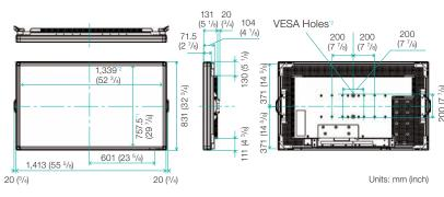
\*1 Screen size \*2 To use a VESA-standard mounting bracket, use M6 screws that are 8 to 10 mm plus the thickness of the bracket.
