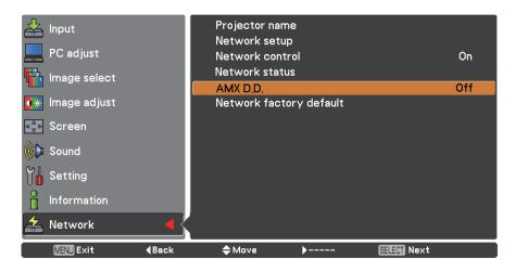
Press <SELECT> button or the ▶ button to select [On] or [Off] to allow the projector to be detected by AMX Device Discovery. For more details, visit http://www.amx.com/.
