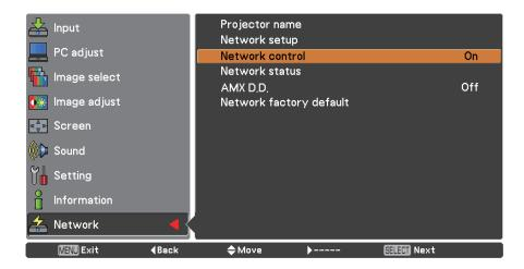
Press <SELECT> button or the ▶ button to select [On] or [Off] with the ▲▼ buttons.
