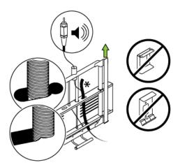
4. Cover cables below the turret base using the split corrugated conduit that is provided with the adjustable height system.
