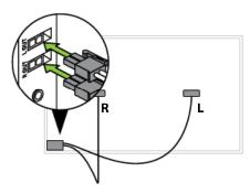
2. Connect the cable from the driver pack on the RIGHT side of the whiteboard to the amplifier connector labeled "L out" for left.
