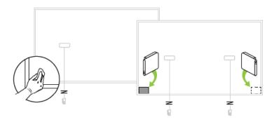
3. Remove the self-adhesive backing from the amplifier.
