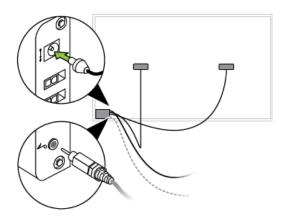
• If installing the whiteboard on an adjustable height mobile stand or adjustable wall mount, do not connect the power or audio input cables to the amplifier until after cable routing is complete. Refer to "Cable routing for adjustable height mobile stand or wall mount options" and "Option: Cable management for adjustable height systems".
