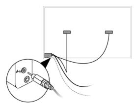
The guest audio input connector is located at the edge of the whiteboard for easy access to temporary connections.
