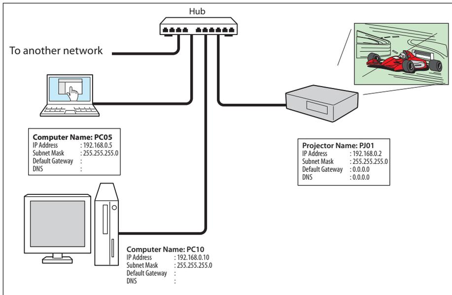
When the projector is connected to the computer directly without hub, the UTP cross cable should be used.
