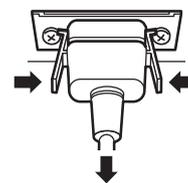
Unplug the AC cord pressing the two knobs.
