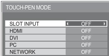
"SLOT INPUT" is displayed when an optional Terminal Board is installed. When a Terminal Board with dual input terminals is installed, "SLOT INPUT A" and "SLOT INPUT B" are displayed.
