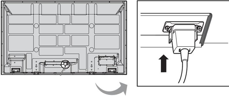
Connecting the plug to the Wall Outlet.
