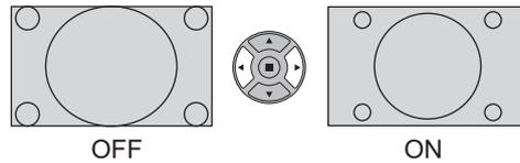
**1:1 PIXEL MODE (2k1k)** When the input signal is a 2k1k signal (2048×1080 / 24p, 2048×1080 / 24sF), the display size is adjusted as follows.
