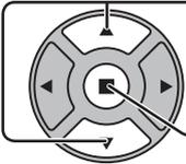
Press to select ON/OFF TIMER SETUP or DAY/TIME SETUP.
