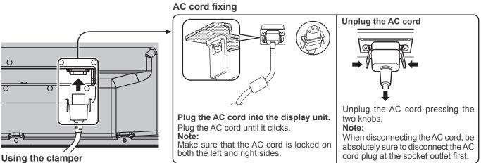
Secure any excess cables with clamper as required. Note:
