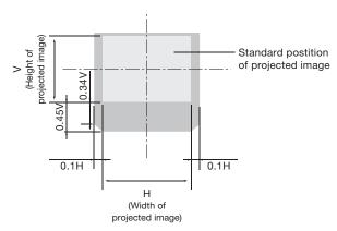
• The ET-DLE055 has a fixed short-focus lens. Therefore, the lens shift function provided in the main unit cannot be used.
