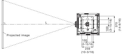
Illustrations show the projector installed using optional ceiling mount bracket ET-PKD120H, optional bracket assembly ET-PKD130B/PKD120B and
