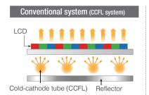
The CCFL system requires the installation of multiple tubes that illuminate in the same way as fluorescent lamps behind the LCD panel. Thus, the display unit becomes thick
