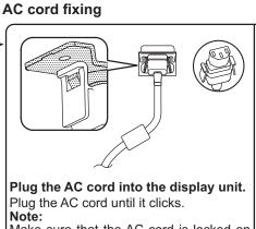
Make sure that the AC cord is locked on both the left and right sides.
