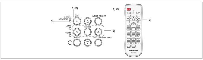
Press the power button <⊕/ |> on the control panel or on the remote control.
