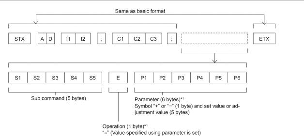
\*1 When transmitting a command which does not need a parameter, the operation (E) and parameter are not necessary.
