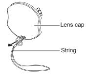
2) Thread the other end of the string through the hole on the bottom of the projector.
