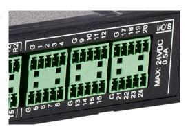
When used as input the voltage has to be below 1 Volt DC to be accepted as LOW, and above 4 VDC (but below 24 VDC) to be accepted as high. The inputs are default high and need to be connected to ground in order to change its state,
