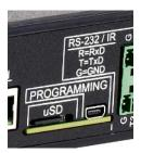
The USB connector needed to connect to the Neets Control – AlFa is of the type mini USB B 5P. You can buy this cable on the web (buy a USB A to Mini USB B 5P).
