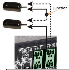
When used as dual IR port: Connect the IR-1 emitter to e.g. T2 (white striped wire) and black wire on IR-1 emitter to IR-2 emitter (white striped wire), and black wire from IR-2 emitter to GND, as shown here above.
