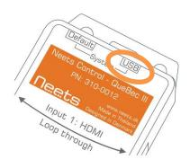
The USB connector needed to connect to the QueBec is of the type USB Mini-B 5P. (A USB A to USB Mini-B 5P connector cable may be purchased online or at many retail stores).
