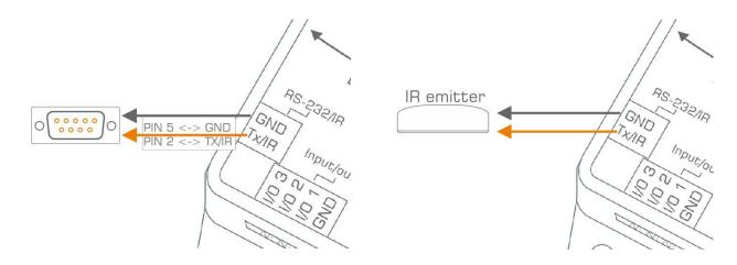
When used as RS-232 transmiter port: Connect the device to Tx/IR and GND, as shown above.
