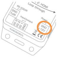
The QueBec accepts only 12 VDC as power source from the supplied power adaptor. If a power adaptor from another manufacturer is used Neets cannot guarantee proper function of the QueBec control system.
