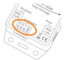
The ports are not potential free; external relays may be required to prevent ground loops.
