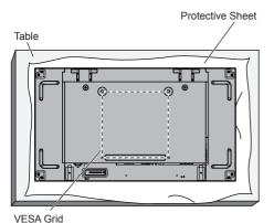
Lay a protective sheet on a flat table, which was wrapped around this Display when it was packaged,
