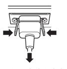
Unplug the connector pressing the two knobs.
