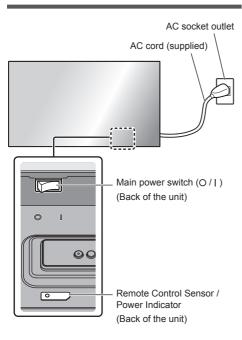
Operate pointing the remote control directly at the unit's Remote Control Sensor.
