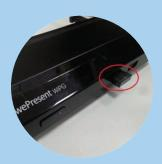
Connect Remove USB Dongle from battery compartment of AirPad and insert into the front USB port of the WiPG-2000
